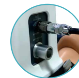
2. Gas inlet Ventilation port
