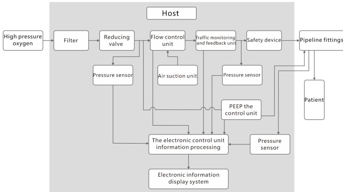
FIGURE 43 T5 Product Structure Diagram
